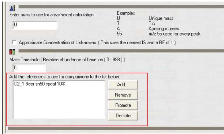
Figure 2. The Data Processing tasks selected for a DP Method using COMPARE are shown in (A). The area at the end of the DP Method where the selected Reference is added is shown in (B). The value for the Mass Threshold in the Reference should match that used in the DP Method originally used to process the sample used in the Reference.
