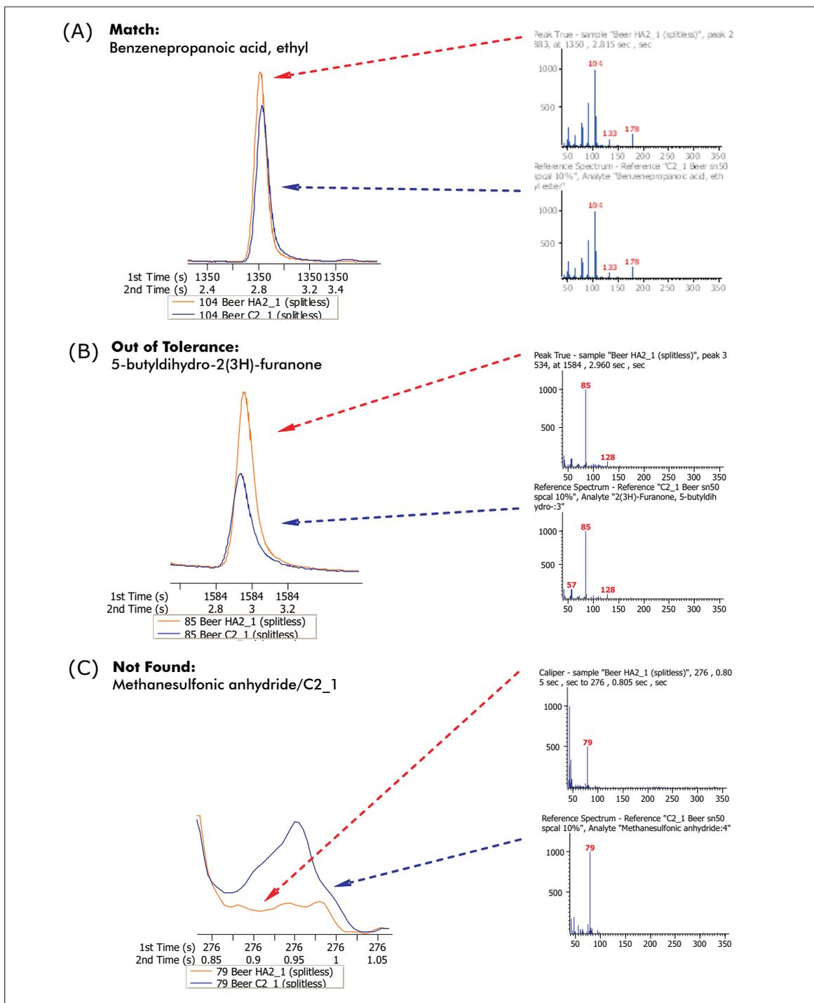
Figure 3.: Examples of chromatograms and spectra for an: (A) Match, (B) Out of Tolerance and (C) Not Found. Red lines indicate association with the Sample and blue lines, the Reference.
