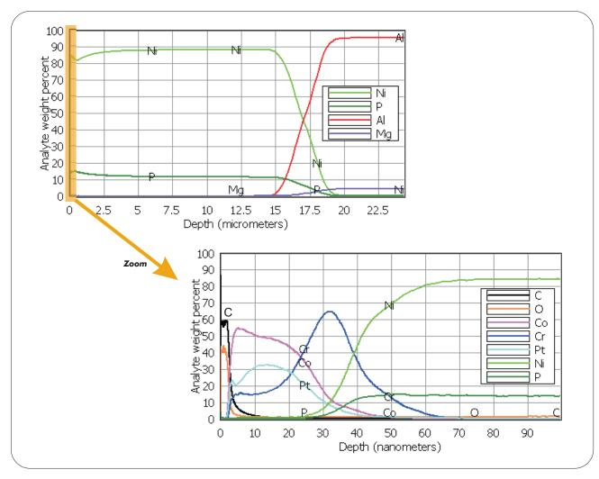
GDS-850A analysis of a commercial hard disk. Layers present include a thin diamond-like carbon protective layer; Pt, Co, and Cr in the magnetic layers; amorphous electroless nickel on an Al-alloy substrate. The zoomed view shows the first 100 nm of analysis.
