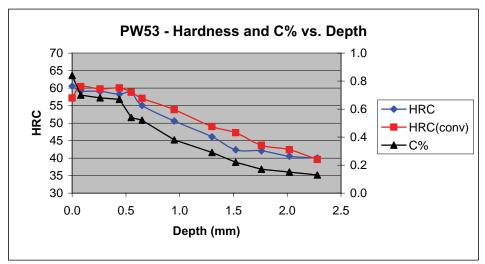
Figure 3: Variation of hardness and carbon concentration versus depth
