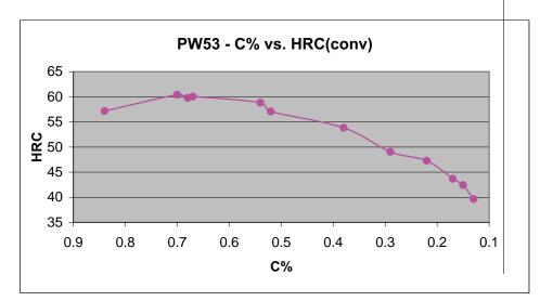
Figure 4: Variation of hardness versus carbon concentration
