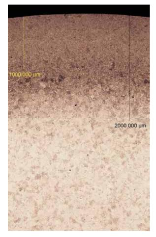
Figure 5: Cross sectional image of sample PW53 50X – 2% Nital
