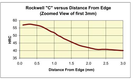
Figure 6: Knoop microhardness analysis on the AMH43 Automatic Microindentation System
