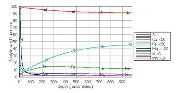
**Homogeneity:** Multiple analyses, obtained on the same sample or different samples, can be compared to determine variation. These analyses can be plotted together and statistical calculations made on values obtained. The plot below shows three replicate analyses on a single sample, and the accompanying tables provide the mean and RSD for each calculated value.
