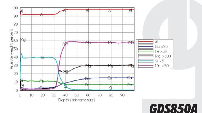
By defining an integration area in the clad and in the core, the software calculates the average chemical composition of both constituents. The clad depth can also be calculated. Calculations are made automatically at the end of the analysis. An example is provided below.
